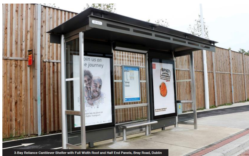
Figure 4-32: Example of a 3-Bay Reliance Cantilever Shelter with Full Width Roof and Half End Panels (Source: JCDecaux)
