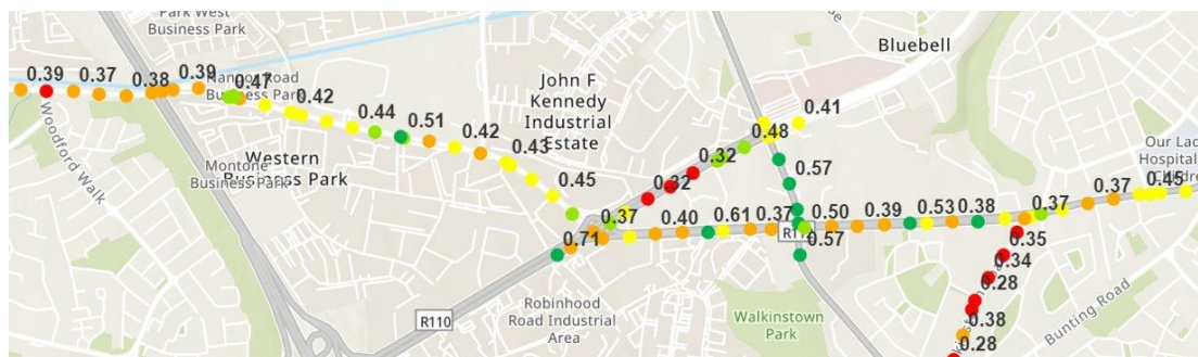
Figure 7-7: Corrected SCRIM Conditions for Proposed Scheme (Clondalkin to Drimnagh). Source: ArcGIS RMO MapRoad (2019 DCC pavement surveys) – Esri UK, Esri, HERE, Garmin, METI/NASA, USGS mapping
