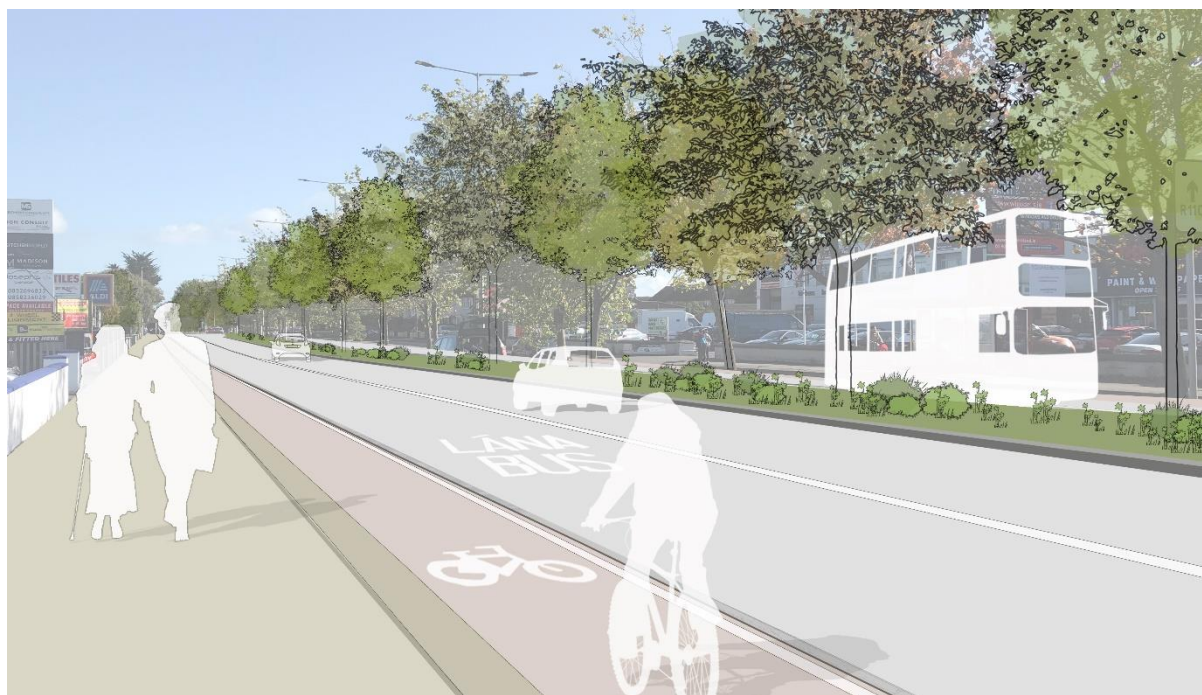
Figure 14-17: Sketch Scheme for Design Intent - Long Mile Road Cycle Track and Enhanced Planting Within Medians
